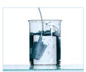
SoftCap® and SoftWrap® sensors can be reliably disinfected and cleaned by dipping into high-level disinfectants solutions.
